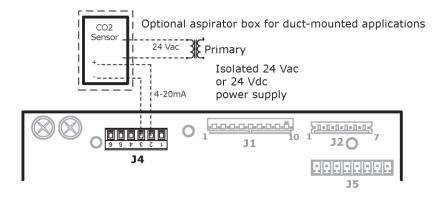
Wiring diagram for #33ZCT55/56C02:
