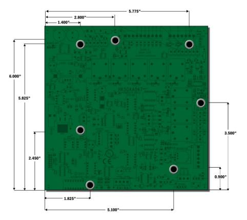
Screw the RTU Open into an enclosed panel using the mounting slots on the cover plate. Leave about 2 in. (5 cm) on each side of the controller for wiring.
