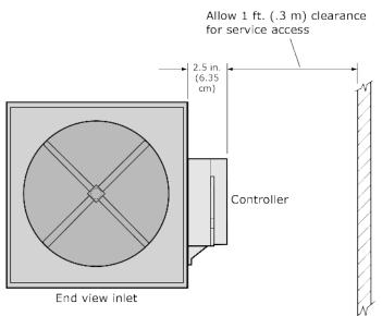
**NOTE** For service access, allow at least 1 foot (.3 m) of clearance between the front of the controller and adjacent surfaces.
