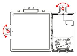
**4** Hold down the actuator damper release button and rotate the actuator clamp in the same direction that closed the damper. Rotate the clamp until it stops, then rotate it back one notch.
