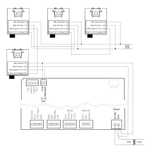
**NOTE** Maintain polarity if using the same power supply for more than one actuator.
