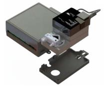
Disconnect the actuator from the controller by inserting a screw driver in the slot on the back of the VVT Zone II and pressing the tab. The actuator cable or an attached extension cable must connect to the controller's **Act Net** port.
